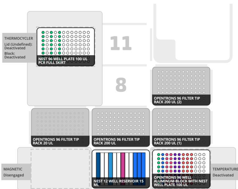
**Figure 2. Opentrons OT-2 deck layout equipped with modules, labware, and Illumina DNA Prep reagents.**
