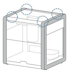
To install onto the OT-2, **slip the key corners on the <u>left hand</u> side of the adaptor** bracket under the sheet metal of the robot as shown below.
