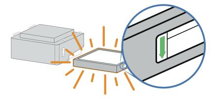
With the help of a 2nd person, lift the main HEPA unit, and place it back on top of the new HEPA filter.
