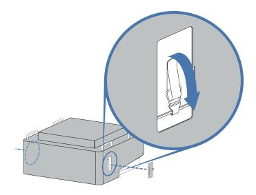
5 Unbuckle the rear filter attachment latch.
