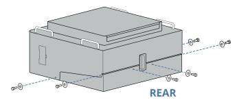
With the help of a 2nd person, lift and remove the main HEPA unit.
