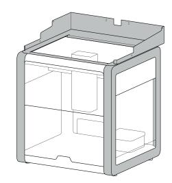
Using the 2.5mm Hex Driver or Allen Key, use the 4 screws included in the Accessory Kit to fasten the adaptor bracket on top of the OT-2. They screw in where the top window screws would usually go. Only use the screws that came with the HEPA module.
