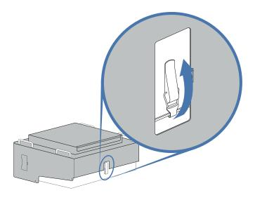
With the help of a 2nd person, pick up and place the complete HEPA unit onto the adaptor bracket (installed on OT-2), so it sits as indicated in the graphic below. Then slide the main HEPA unit back to its furthest rear position.
