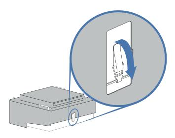
Place the new filter next to the HEPA unit ensuring the arrow indicating airflow is pointing down towards the ground.
