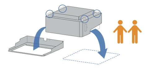
Install the adaptor bracket onto the top of the OT2. This can be done by one person.
