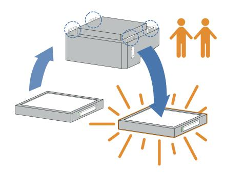
Re-buckle the latches and replace the pop-out covers on either side of the unit to cover the filter release latches.
