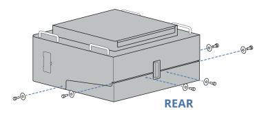
With the help of a 2nd person lift the main HEPA unit, removing it from the adaptor bracket. Set the main HEPA unit aside on an accessible work surface.
