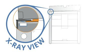
Once the left side key corners are correctly placed, the adaptor bracket should sit flat on top of the robot and not wiggle around.
